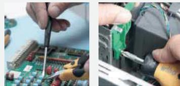
**Sensitive, electronic components can be damaged even at a very low voltage.**
